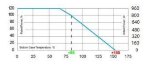
Derating (thermal resist.) SUP800: 8.47W/K (0.12 K/W)
