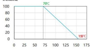
Derating (thermal resist.) RHP150: 1.76 W/K (0.57 K/W)
