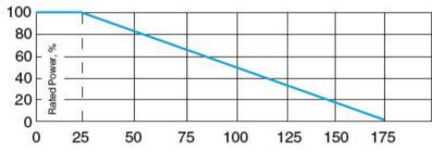
Derating (thermal resist.) LXP100 /LXP100 L: 0.66 W/K (1.5 K/W)
